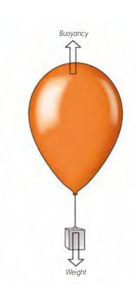
The other forces applied to the balloon are the friction of air on the envelope (if the balloon has vertical speed), and its weight.
