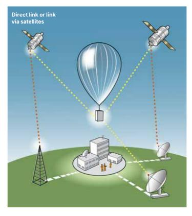
Balloons have gondolas which are constantly connected to a ground control centre. These gondolas are used to operate onboard actuators to release either gas or ballast. This makes it possible to control the ascent or descent of the balloon from the ground.
